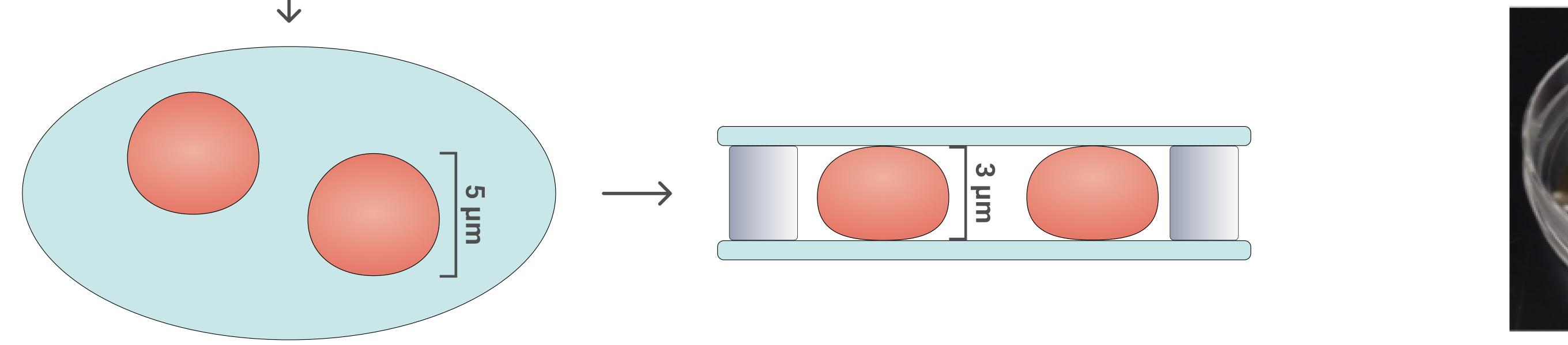
Schematic explanation of the confining system (on the left). The confining system consists of the micropillars (enlarged right in red) on top of the confining PDMS cylinder placed in the middle of the device with magnets (top image). The entire confining device in a petri dish, micropillars facing down. The device is fixed using magnets engaged to a metal ring below the dish (bottom image).
