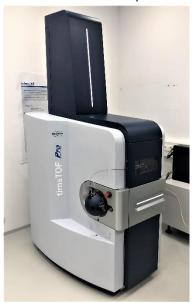
A new mass spectrometer timsTOF Pro from Bruker Daltonics was installed in the Structural mass spectrometry core facility. The mass spectrometer is mostly used for high throughput shotgun proteomics, hydrogen-deuterium exchange and covalent labelling experiments, and native mass spectrometry with ion mobility separation. The high sensitivity and sequencing speed allow identification of more peptides and their post-translational modifications.
